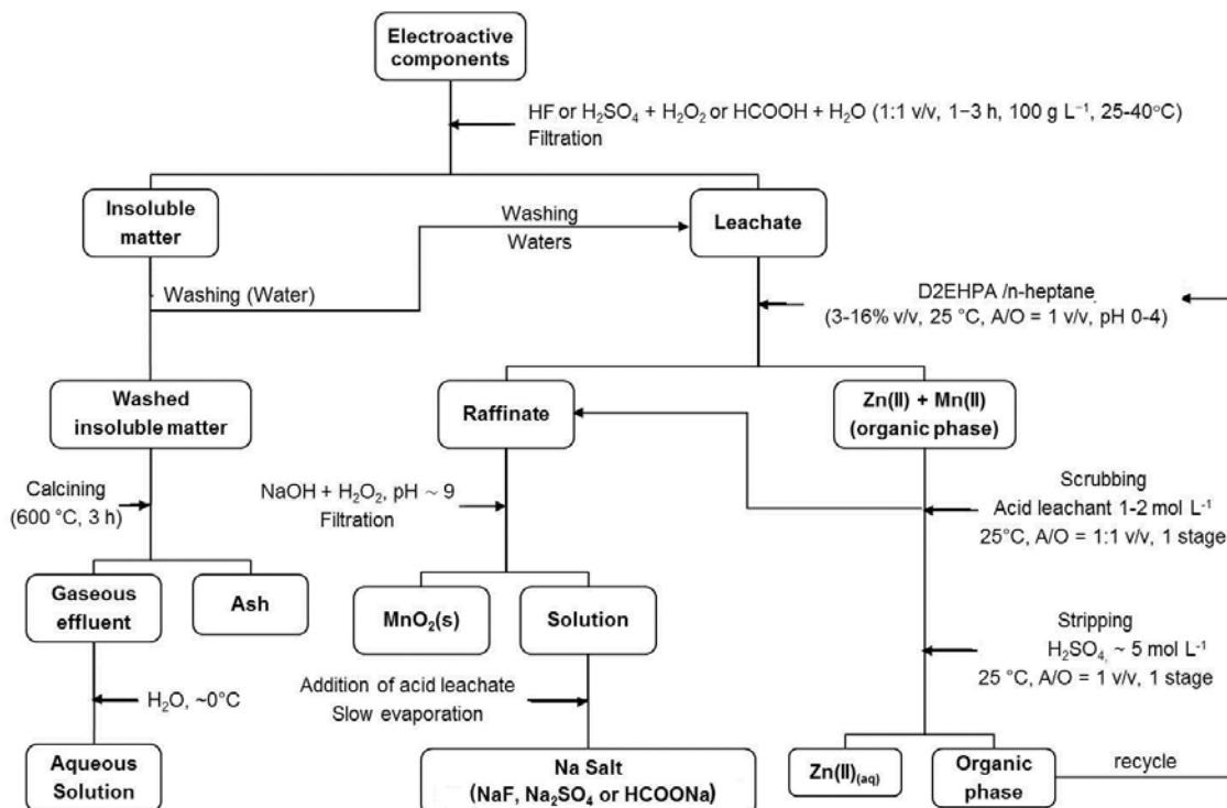
**Figure 1S.** General scheme for the recovery of zinc and manganese from spent zinc-MnO<sub>2</sub> dry cells after acid leaching in the presence of a reductant
