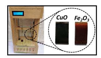
Dip-coater machine to produce high quality thin films.
