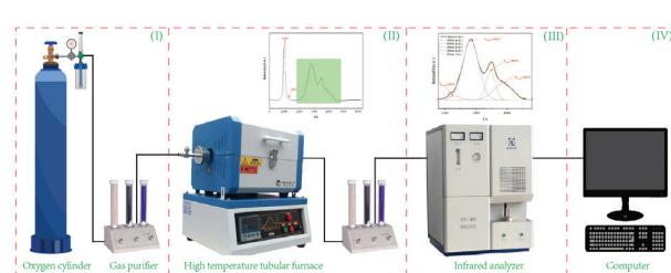
TPO-IR method was used for rapid determination of sulfur species in solid minerals. During the TPO process, sulfur species in minerals are oxidized or pyrolyzed to form sulfur dioxide which is detected by infrared detector. The content of sulfur species was quantified by fitting curve information.
