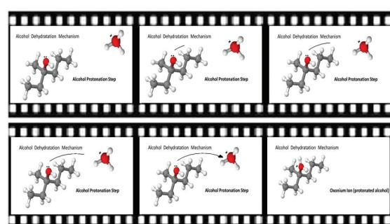
Sequential images showing the first step of the alcohol dehydration mechanism - alcohol protonation step.
