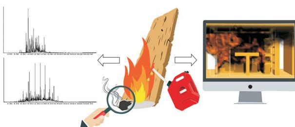
The use of GC-MS in the identification of arson-derived accelerants and computer simulation using FDS to verify whether fire damage is compatible to occur naturally or only with the use of accelerant.
