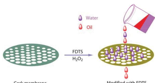
Fabrication of the FDTs-modified cork membrane and separation of oil/water mixtures.
