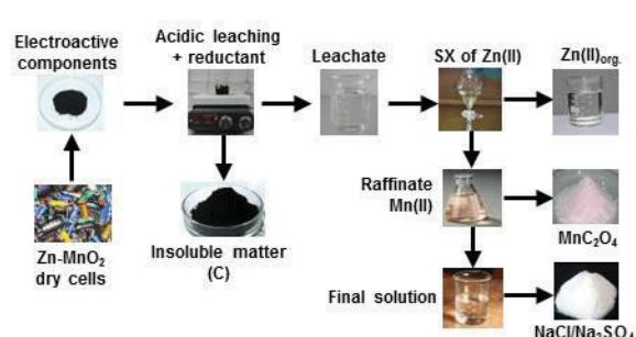
Efficient leaching of spent zinc-MnO<sub>2</sub> dry cells under mild experimental conditions using strong acids. Zn(II) was preferably extracted over Mn(II) by TBP or Cyanex 923.
