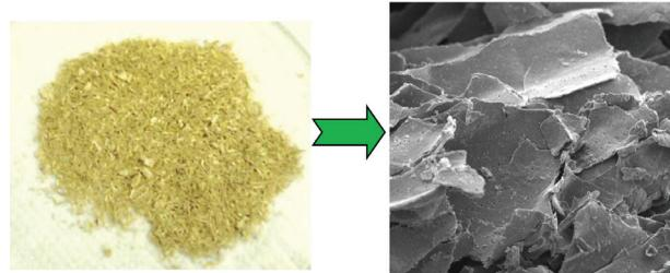
Sugarcane bagasse fibers modified superficially through the carboxymethylation process - *in natura* and MEV image - that were used to adsorb contaminants in biodiesel from soybean oil.
