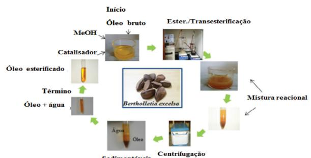
Schematic diagram showing the homogeneous esterification and transesterification steps of Brazilian nut oil (*Bertholletia excelsa*).
