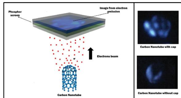
The phosphor screen integrated in the field emission microscope system allows: to evaluate if nanotubes have cap; estimate the area of emission; estimate the amount of nanotubes that are emitting; compare different emitters and study the emission behavior.
