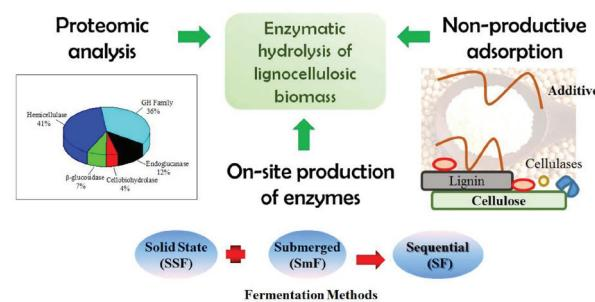
Schematic illustration of the potential strategies to address the current limitations of the enzymatic hydrolysis of lignocellulosic biomass: the production of enzymes on-site, the use of secretome analysis for enzymatic characterization and some approaches to reduce unproductive adsorption of enzymes onto lignin.
