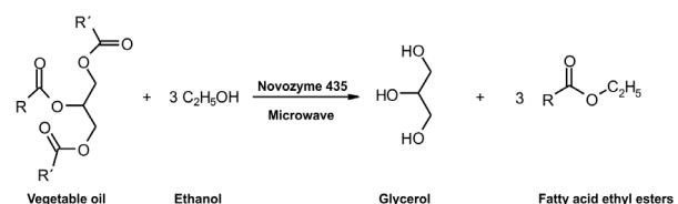
Complete transesterification of soybean oil catalyzed by Novozyme 435 under microwave.
