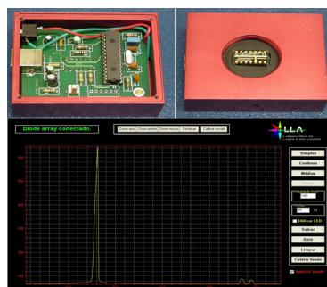
Picture of the light intensity acquisition apparatus developed including: the electronic control circuit, linear diode array and software graphics interface with a Hg lamp spectrum displayed.
