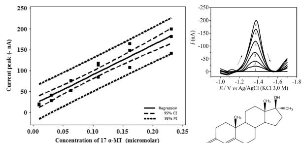
This study presents the in-house validation of a new voltammetric methodology for 17 $\alpha$ -MT analysis in natural water. The methodology exhibited selectivity, linearity, accuracy and precision.
