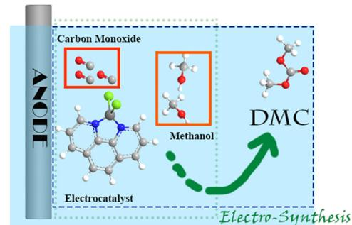
Dimethyl carbonate (DMC) is viewed as an environmentally benign intermediate because of its negligible eco-toxicity and its versatile chemical applications. In this paper, a novel homogeneous electrocatalyst based on Cu(Phen)Cl<sub>2</sub> was used for electrocatalytic oxidative carbonylation of methanol to DMC.
