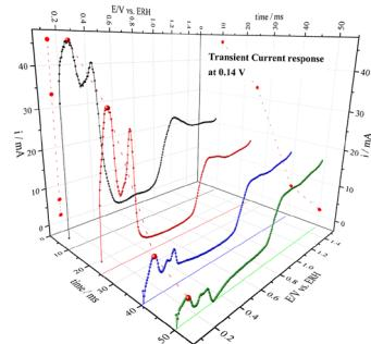
Cyclic voltammogram profile of platinum in acid media obtained by *Staircase Sweep Voltammetry (SCV)*. The data displays the current recorded at different periods during each step comprising the SCV signal.
