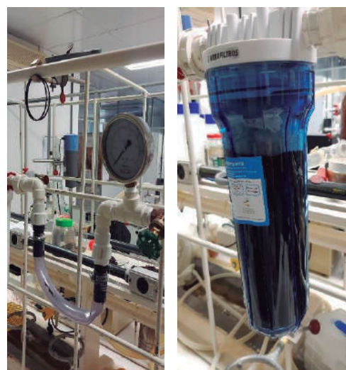
Figure 1 Prototyping of the biosorption of metals endocarp of macauba
