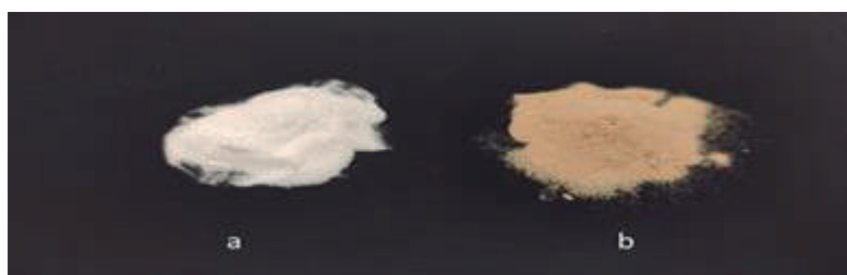
Figure 1: Photograph of PA12 powder before (a) and after (b) AgNP incorporation.
