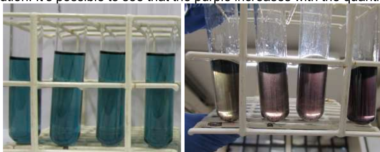
Figure 1. A) Left to right: ethanol samples mixed with 0,3%, 0,5%, 0,6%, 0,9% methanol. After, all solutions were mixed with potassium dichromate solution. B) Left to right: ethanol mixed with 0,3%, 0,5%, 0,6%, 0,9% methanol. After, potassium dichromate and chromotropic acid solution were added to all the solutions.
