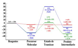
**Figure 2.** Energy profile for  $CuO^+$  and  $CH_4$  reaction mechanisms.
