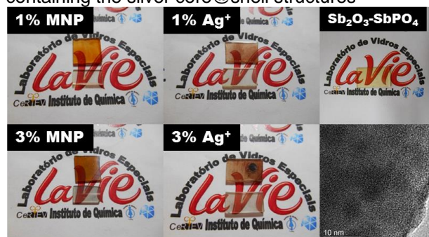
Figure 1. Images of glass synthesized after and before the heat treatment above T_g and TEM of 1% MNP without heat treatment.
